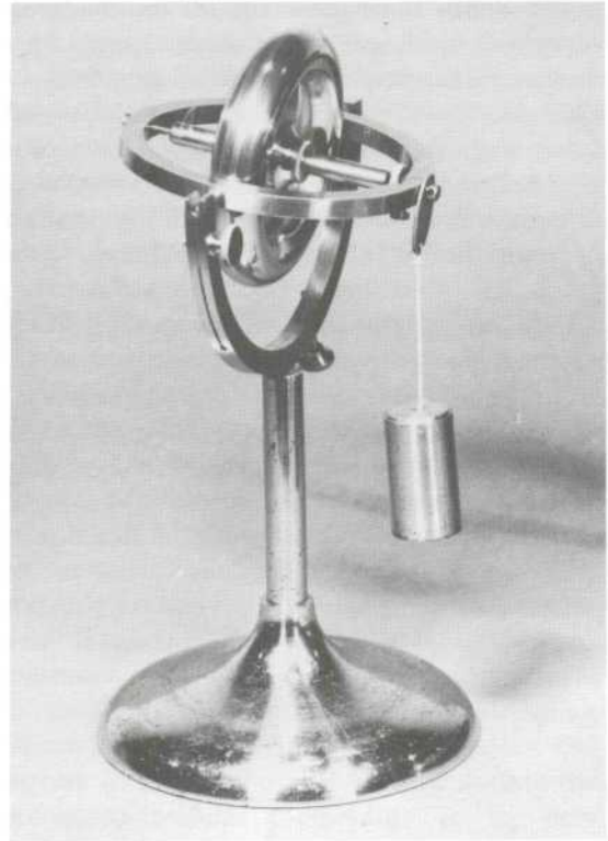
Plate 4.3 The gyro 'precesses' about a vertical axis when a weight is hung from the inner ring.
