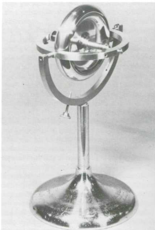
Plate 4.2 A scientific gyroscope consists of a wheel mounted in gimbal rings.
